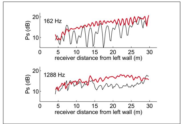
Figure 1. Reflected pressure level (arbitrary reference) for two example one-third octave frequencies as a function of receiver distance. — Corrugated ceiling; — Flat ceiling.
