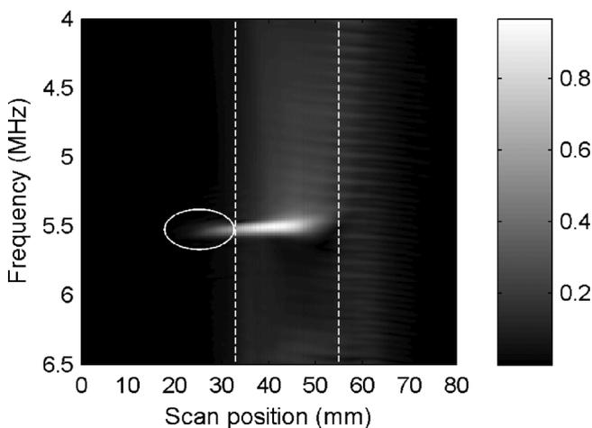
FIG. 2. Spatial spectrogram showing reflected ultrasonic field for an angle of incidence of 30°. Backward displaced frequencies (circled) observed in the vicinity of 5.51 MHz. Specular beam shown with dashed lines.
