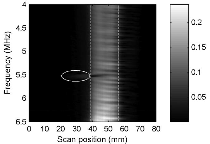
FIG. 3. Spatial spectrogram showing transmitted ultrasonic field for an angle of incidence of 30°. Backward displaced frequencies (circled) observed in the vicinity of 5.52 MHz. Specular beam shown with dashed lines.
