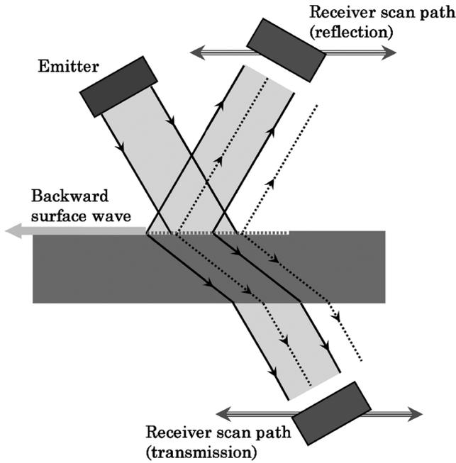
FIG. 1. Illustration of experimental setups for measurement of backward beam displacement in reflection and transmission. Specular beams shown in dotted lines and backward shifts shown in solid lines.
