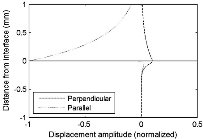
FIG. 4. Particle displacement amplitudes calculated for a 5.5 MHz Scholte–Stoneley wave propagating on a water–brass interface. Displacement perpendicular to the interface shown with dashed lines and displacement parallel to the interface shown with dotted lines. Displacement amplitudes are observed to decrease dramatically with penetration depth in the solid (negative distance from interface).
