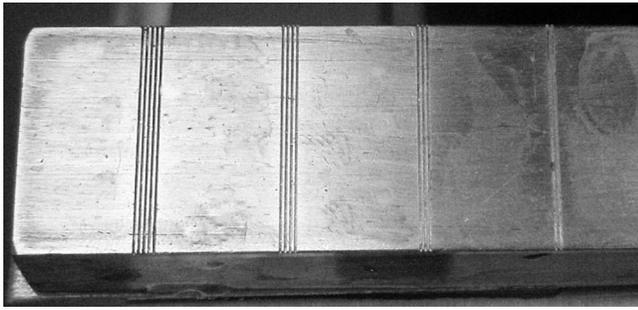
FIG. 5. Photographic picture of a brass sample with rectangular grooves engraved of 0.0254 cm deep and wide. The grooves are organized in sets of 2, 3, 4 and 5 grooves
