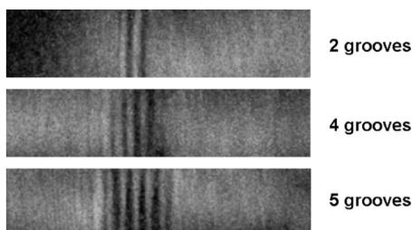
FIG. 6. Bragg images of the sets of 2, 4 and 5 grooves as shown in Fig. 2.
