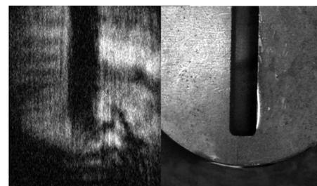
FIG. 4. Bragg image (left) and photographs image (right) of a 4 mm wide slit in a circular brass disk of 2 mm thickness. The disk is placed on a damping material to make sure only reflection from the brass disk is possible. The slit and the disk edge are clearly visible on the Bragg image.
