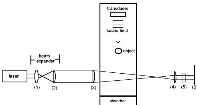
FIG. 2. Experimental setup used in the traditional acoustic Bragg diffraction experiment.
