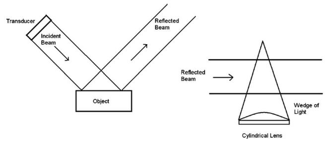
FIG. 3. Bragg imaging from a reflected acoustic beam.
