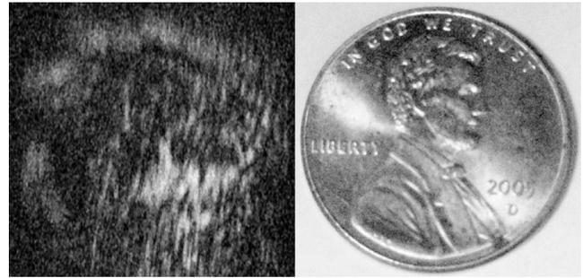
FIG. 7. Bragg image of a coin.
