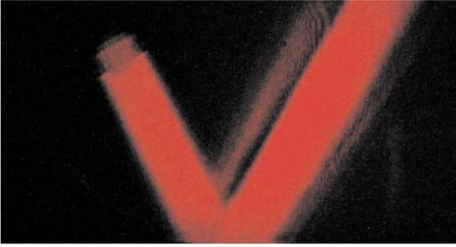
FIG. 2. (Color online) Acousto-optic schlieren picture of the Schoch effect (accompanied by null strip in between specular and nonspecular reflected beams) in the absence of an acoustic barrier.
