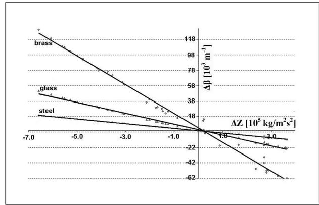
Figure 3. The same procedure was followed as in Figure 2, but for different materials of the solid plate (resembling a container skin) and only for experimentally existing liquids. Note that the results follow straight lines and the direction of each straight line is a function of the solid under consideration.
