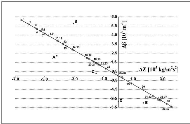
Figure 2. The inhomogeneity difference  $\Delta\beta = \beta - \beta_0$  as a function of the impedance difference  $\Delta Z = Z - Z_0$ . The results for the stainless steel plate, in the case of  $A_1$  Lamb wave stimulation, for 'liquid 1' = water and 'liquid 2' listed in Table I. The codes corresponding to the different liquids are tagged.
