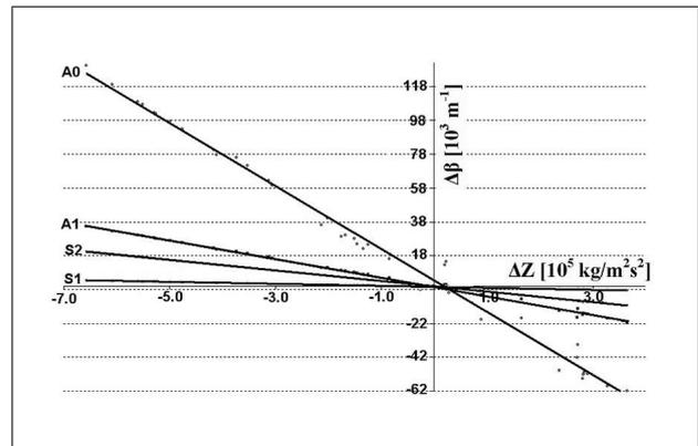
Figure 4. A brass plate is considered under the same circumstances as in Figure 2 and Figure 3, though for different Lamb waves. The direction depends on the type of Lamb wave.
