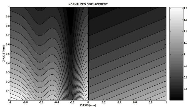
Figure 8. A filled contour plot of the normalized total displacement  $|u|$  of the new kind of surface wave (the one of Figure 7) as a function of  $z$  and the propagation distance  $x$ .
