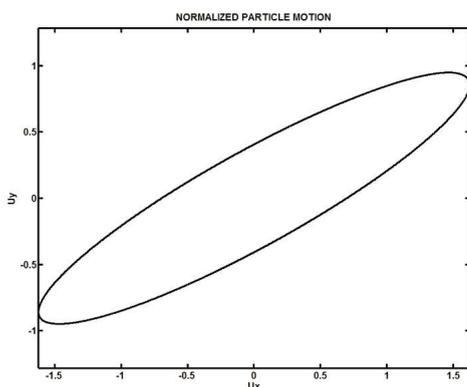
Figure 10. The particle normalized displacement in the solid for the new kind of surface wave of Figure 9 at  $[x, z] = [0, 0]$ , depicted over 1 period of time. Note that this corresponds to nearly linear elliptical polarization, and differs from the polarization of a leaky Rayleigh wave (see Figure 6).
