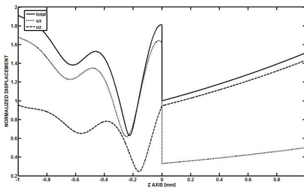
Figure 7. The normalized amplitude profile of the new kind of surface wave at 5 MHz. The angle of incidence is 19.01 degrees, with inhomogeneity  $-1269.39/m$ . The dotted line corresponds to  $|u_x|$ , the dashed line to  $|u_z|$ , while the solid line corresponds to  $|u|$ .
