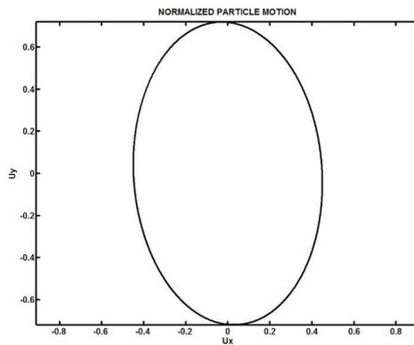
Figure 6. The normalized particle displacement in the solid for the leaky Rayleigh wave of Figure 5 at  $[x, z] = [0, 0]$ , depicted over 1 period of time. It is clear that this corresponds to elliptical polarization.
