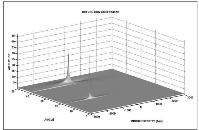
Figure 2. The amplitude of the reflected waves for different inhomogeneities and for different incidence angles on a brass/water interface. Note the appearance of two peaks. The one at an angle of 44.05 degrees is the Rayleigh peak, whereas the one at an angle of 19.01 degrees corresponds to the new kind of surface waves.
