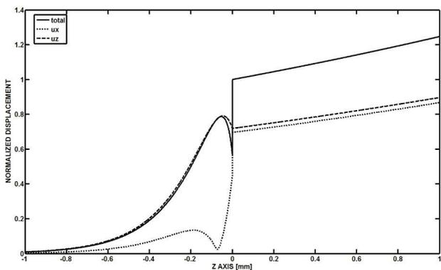
Figure 3. Normalized amplitude profile of a Rayleigh wave at 5 MHz. The angle of incidence is 44.05 degrees, with inhomogeneity  $-317.27/m$ . The dotted line corresponds to  $|u_x|$ , the dashed line to  $|u_z|$ , while the solid line corresponds to  $|u|$ .
