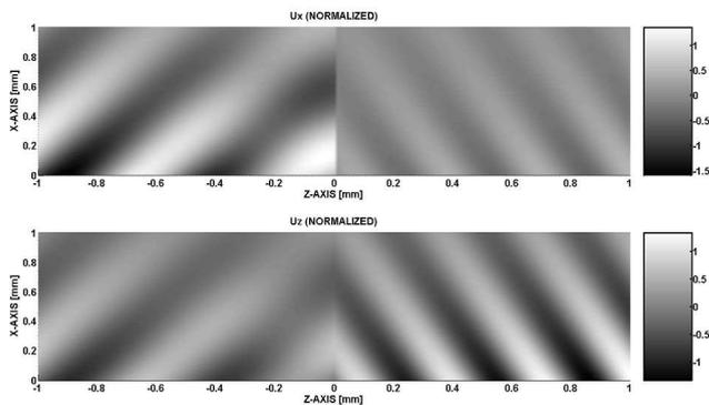
Figure 9. The real part of the normalized displacement ( $u_x$ : top;  $u_z$ : bottom) as a function of  $z$  and the propagation distance  $x$  for the new kind of surface wave of Figure 8. The new kind of surface wave is elliptically polarized (almost linearly).
