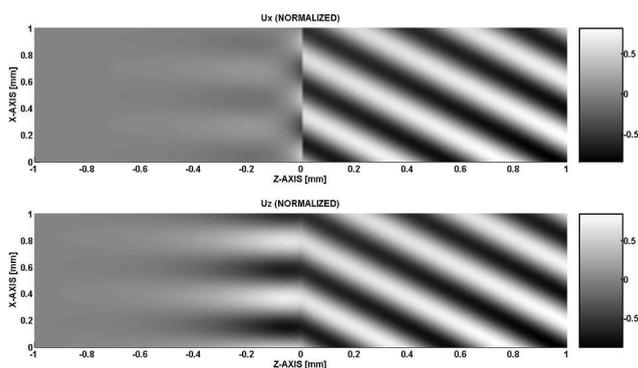
Figure 5. The real part of the normalized displacement ( $u_x$ : top;  $u_z$ : bottom) for time  $t = 0$ , as a function of  $z$  and the propagation distance  $x$  for the leaky Rayleigh wave of Figure 4. The leaky Rayleigh wave is elliptically polarized, which is a well known feature of such surface waves.
