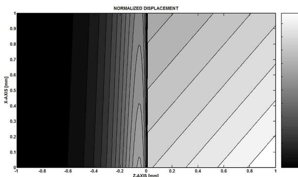
Figure 4. A filled contour plot of the normalized total displacement  $|u|$  of a Rayleigh wave (the one of Figure 3) as a function of  $z$  and the propagation distance  $x$ .
