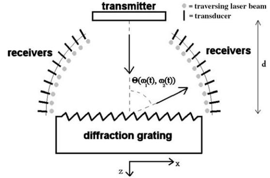
Fig. 1. A schematic of the ‘thought device’, based on sound normally incident on a diffraction grating and diffracted into several directions. A discrete number of omni-directional transducers is placed at constant distance and different angles. In front of each transducer there is a laser beam traversing the sound beam in order to obtain the phase propagation direction as distinguished from the energy propagation direction.
