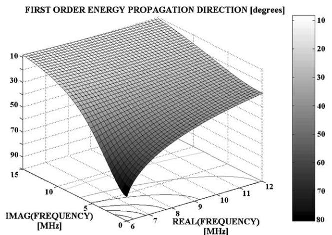
Fig. 5. The first order energy propagation direction as a function of the complex frequency for normal incident sound. The lines on the horizontal surface are projected equi-amplitude lines. Comparison of Fig. 4 reveals that for a given phase propagation direction and energy propagation direction, there corresponds only one couple  $(\omega_1, \omega_2)$ . The reason is that each equi-amplitude line here does not cross a equi-amplitude line of Fig. 4 twice.
