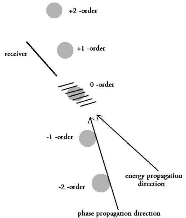
Fig. 2. A close up of the omni-directional transducers of Fig. 1, with attention to the diffraction direction of the traversing laser light. The difference between energy propagation direction and phase propagation must be measurable with this principle.
