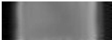
**FIGURE 3.** Reflected-beam pattern for an aluminum sample. No fringes are visible.
