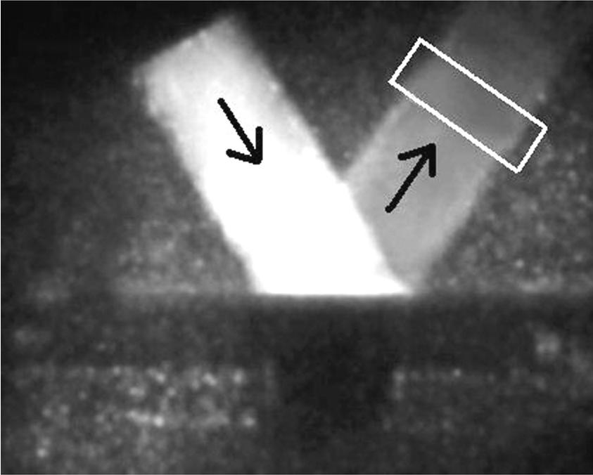
**FIGURE 2.** 2.5-cm-wide 10-MHz ultrasonic beam incident and reflected on an aluminum block. From the visualized reflected beam we always extract the area on the picture denoted by the white rectangle for studying the reflected-beam pattern.
