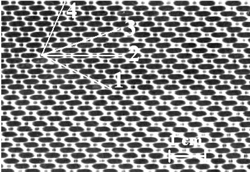
**FIGURE 9.** Definition of the direction 1 ( $-25^\circ$ ), 2 ( $0^\circ$ ), 3 ( $19^\circ$ ), and 4 ( $65^\circ$ ) on the upper surface of a PPS five-harness satin-weave-fabric carbon-fiber-reinforced composite.
