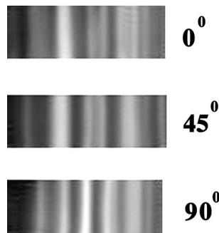
**FIGURE 7.** Reflected-beam pattern for a  $[0^\circ]_8$  stacked glass-epoxy laminate with layers reinforced with unidirectional composite such as in Fig. 5.
