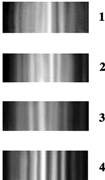
**FIGURE 10.** Reflected-beam pattern along the directions as defined in Fig. 9 for a  $[0^\circ]_8$  stacked laminate with layers as described in Fig. 8. The upper layer has a direction equal to the layer shown photographically in Fig. 9.
