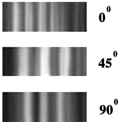
**FIGURE 8.** Reflected-beam pattern for a  $[0^\circ/90^\circ]_{2s}$  stacked glass-epoxy laminate with layers reinforced with unidirectional composite such as in Fig. 5.
