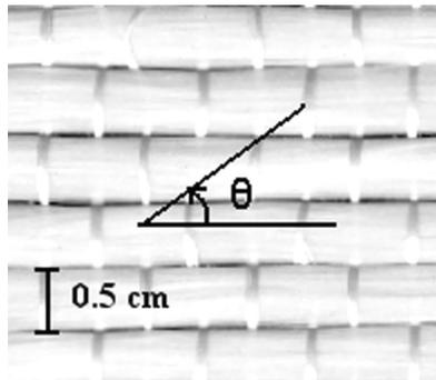
**FIGURE 6.** Photograph of the fibers that are used in manufacturing the unidirectional glass-fabric-reinforced epoxy samples. The width of the warp bunches (horizontal) is 5 mm. The angle  $\theta$  is shown and corresponds to the angles denoted in Figs. 7 and 8.
