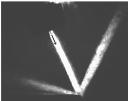
FIG. 4. Schlieren image of a 6-mm-wide ultrasonic beam incident upon a brass reflector at an angle of incidence slightly larger than  $22.5^\circ$ ; besides a diffracted beam near the interface, a sound beam is visible which propagates along the interface, being scattered in the forward direction at the extremity of the sample.
