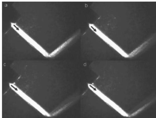
FIG. 7. Schlieren pictures of a 6-mm-wide bounded beam, incident at angles in the vicinity of  $45^\circ$ . Changes of the reflected beam's profile are visible.
