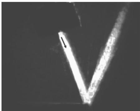
FIG. 5. Schlieren image of a 6-mm-wide ultrasonic beam incident upon a brass reflector at  $22.5^\circ$ ; a sound field is visible on the interface in the backward direction, being scattered in the forward direction at the extremity of the sample. This is evidence that it is a Scholte–Stoneley wave.
