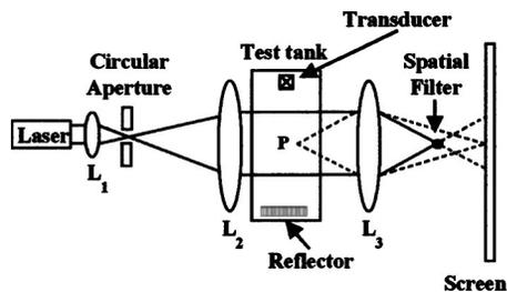
FIG. 1. Experimental setup of the schlieren optical system.
