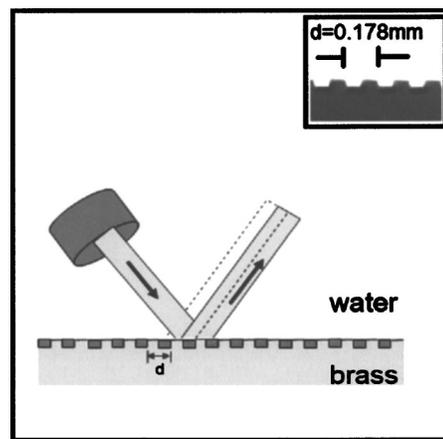
FIG. 2. Schematic arrangement of the transducer and grating shown in Fig. 1. The inset is a photograph of the ruled section of the grating.
