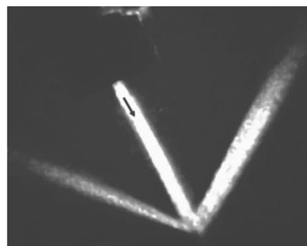
FIG. 3. Schlieren image of a 6-mm-wide ultrasonic beam incident upon a brass reflector at a certain angle of incidence different from any critical angle.
