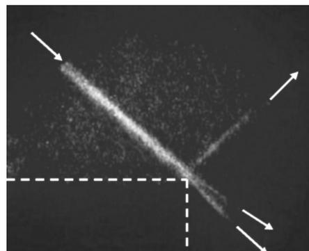
FIG. 8. Incidence of 6 MHz, 0.6-cm-wide bounded beam on brass.  $W \approx 0.9$  cm,  $\Delta \approx 0.8 W$  (Schlieren picture). The dashed lines show where the plate is situated in the experiment. The arrows show the sound propagation direction.
