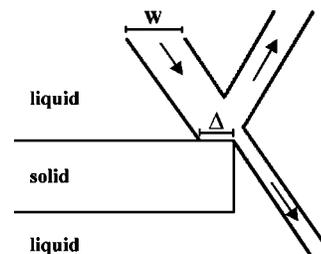
FIG. 2. Definition of  $\Delta$ : the distance between the first beam edge and the plate edge and  $W$ : the horizontal physical width of the beam.
