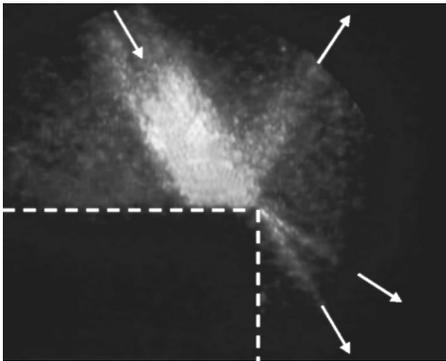
FIG. 4. Incidence of 3 MHz, 2.5-cm-wide bounded beam on aluminum.  $W \approx 2.9$  cm,  $\Delta \approx 0.78 W$  (Schlieren picture). The dashed lines show where the plate is situated in the experiment. The arrows show the sound propagation direction.
