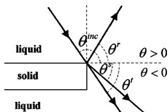
FIG. 1. Definition of the different angles  $\theta^{inc}$ ,  $\theta^r$ ,  $\theta^s$ , and  $\theta^t$ . The angles are measured from the horizontal axis left from the plate. The positive angles are anticlockwise, whereas the negative angles are clockwise.
