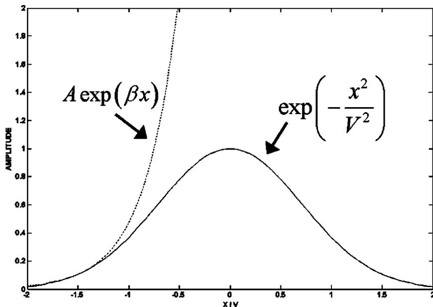
FIG. 7. The edges of a Gaussian beam have a profile that is relatively similar to that of an inhomogeneous wave. This is probably the reason why the edges of a Gaussian beam stimulate the leaky Rayleigh waves. The  $x$  axis is directed along the wave front. The value  $\beta$  is called the inhomogeneity of the accompanied inhomogeneous wave.
