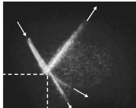
FIG. 6. Incidence of 6 MHz, 0.6-cm-wide bounded beam on aluminum.  $W \approx 0.7$  cm,  $\Delta \approx 0.6 W$  (Schlieren picture). The dashed lines show where the plate is situated in the experiment. The arrows show the sound propagation direction.
