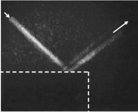
FIG. 9. Incidence of 6 MHz, 0.6-cm-wide bounded beam on brass.  $W \approx 0.9$  cm, far from the edge, the Schoch phenomenon is visible. (Schlieren picture). The dashed lines show where the plate is situated in the experiment. The arrows show the sound propagation direction.
