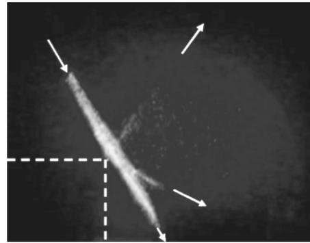
FIG. 5. Incidence of 6 MHz, 0.6-cm-wide bounded beam on aluminum.  $W \approx 0.7$  cm,  $\Delta \approx 0.2 W$  (Schlieren picture). The dashed lines show where the plate is situated in the experiment. The arrows show the sound propagation direction.
