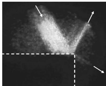
FIG. 3. Incidence of 3 MHz, 2.5-cm-wide bounded beam on aluminum.  $W \approx 2.9$  cm,  $\Delta \approx W$  (Schlieren picture). The dashed lines show where the plate is situated in the experiment. The arrows show the sound propagation direction.
