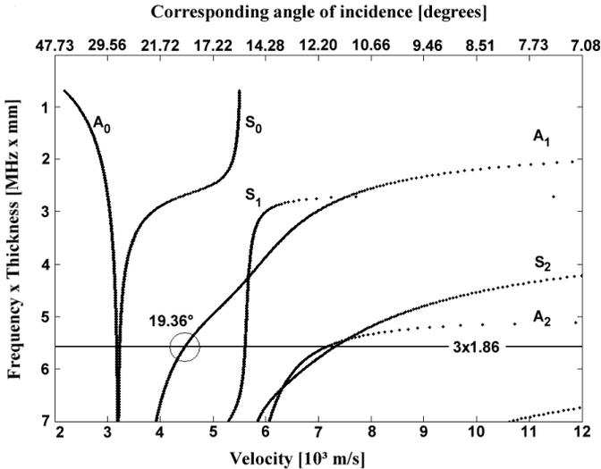
Fig. 2. Dispersion curves for the glass plate under consideration. It is seen that an angle of incidence of 19.36° corresponds with the stimulation of the  $A_1$  mode when a 3 MHz ultrasonic beam is incident on a plate of 1.86-mm thickness.
