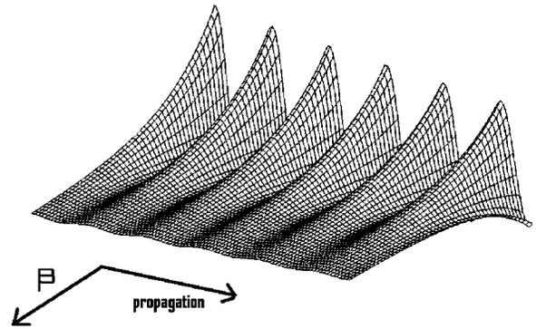
FIG. 3. An infinite inhomogeneous wave (undamped). The amplitude along the wave front decays exponentially down the inhomogeneity vector  $\boldsymbol{\beta}$  [according to its definition in (4)]. The amplitude remains constant along the propagation direction.
